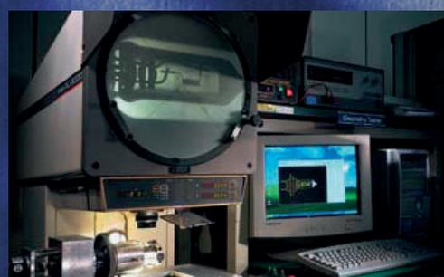
Bulb Geometry Test Equipment
