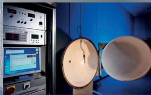
Automatic Initial Photometry Test Equipment
