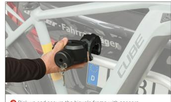
3 Pick up and secure the bicycle frame with spacers. The spacers are lockable.
